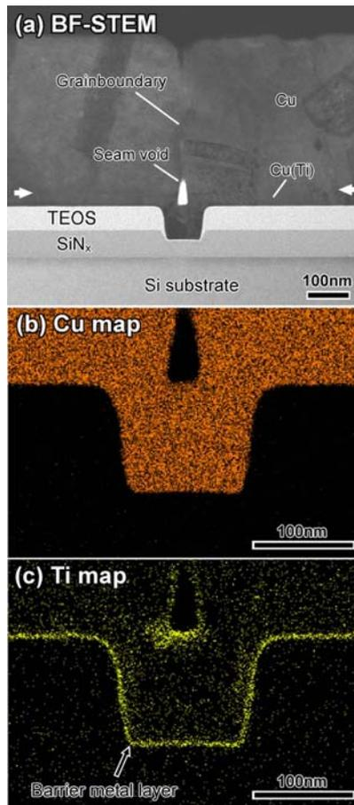
FIG. 1. Cross-sectional STEM-EDS images of the interconnect fabricated by embedding the Cu(Ti)/Cu films into the trench; (a) bright-field STEM image, and EDS elemental mapping image of (b) copper and (c) titanium.
