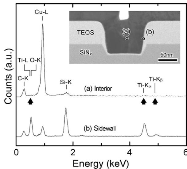
FIG. 2. EDS spectrum profiles obtained from the regions of (a) the trench interior and (b) the oxide interface, which are marked by circles in the STEM image inserted in the figure.
