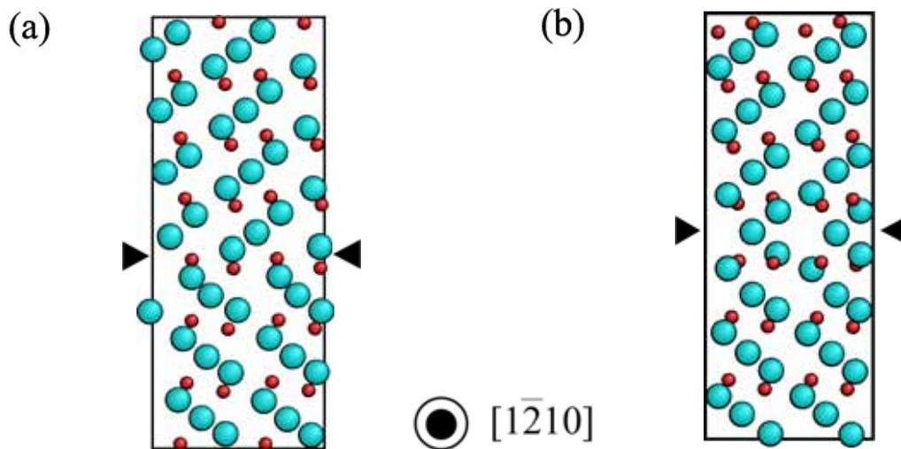
FIG. 2. Theoretically predicted  $\Sigma$ 13 grain boundary structures. Arrowed regions are the grain boundary.(a)Al-terminated structure (b) O-terminated structure [4].
