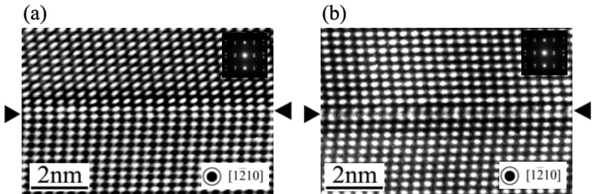
FIG. 1. HRTEM images of (a) pristine and (b) Y-doped  $\Sigma$  13 grain boundary. Arrows indicate the position of grain boundaries.
