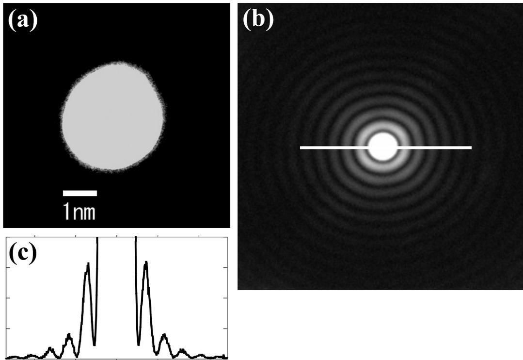
Fig. 1 : (a)The TEM image of the selected area aperture effectively about 3 nm in diameter.
