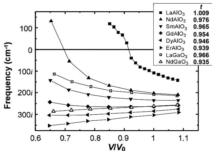
FIG. 2. Frequencies of R point soft mode versus normalized volume for various compounds
