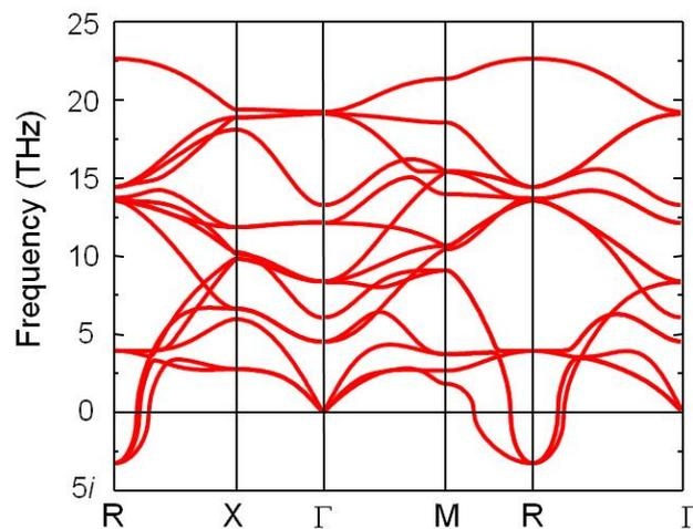
FIG. 1. Calculated phonon dispersion relation of LaAlO<sub>3</sub> in cubic perovskite phase
