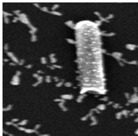
Fig 3 The deposition of silver nanoparticles on a MWCNT is used to anchor the
