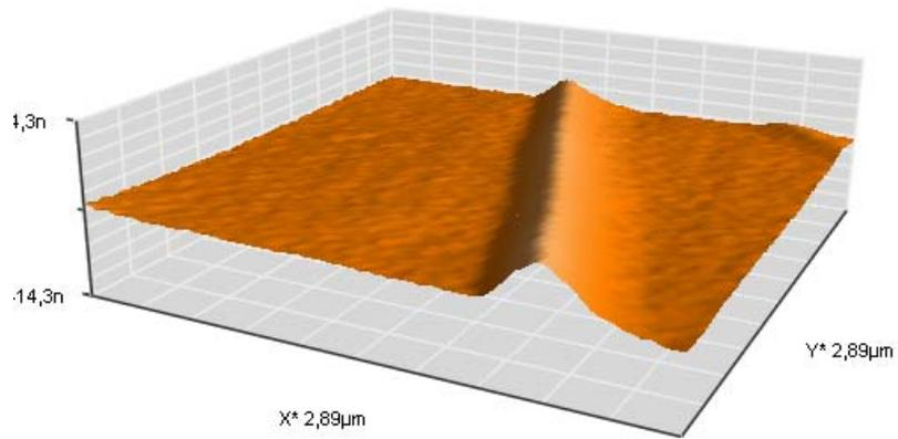
Fig 1 AFM image of pleated graphite
