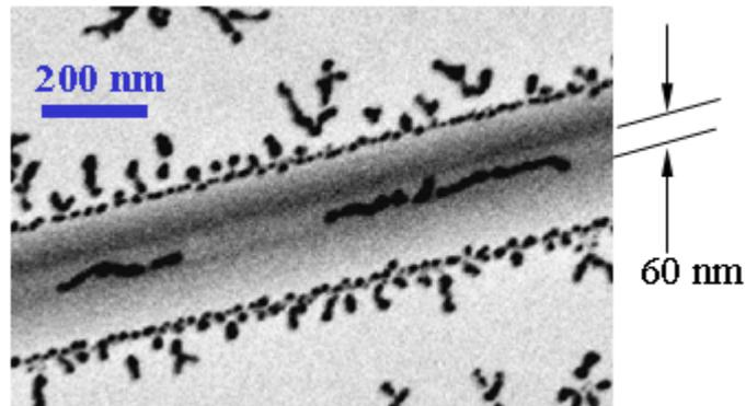
Fig 2 TEM image: The deposition of silver nanoparticles on pleated graphite are forced to grow linearly in nanorods
