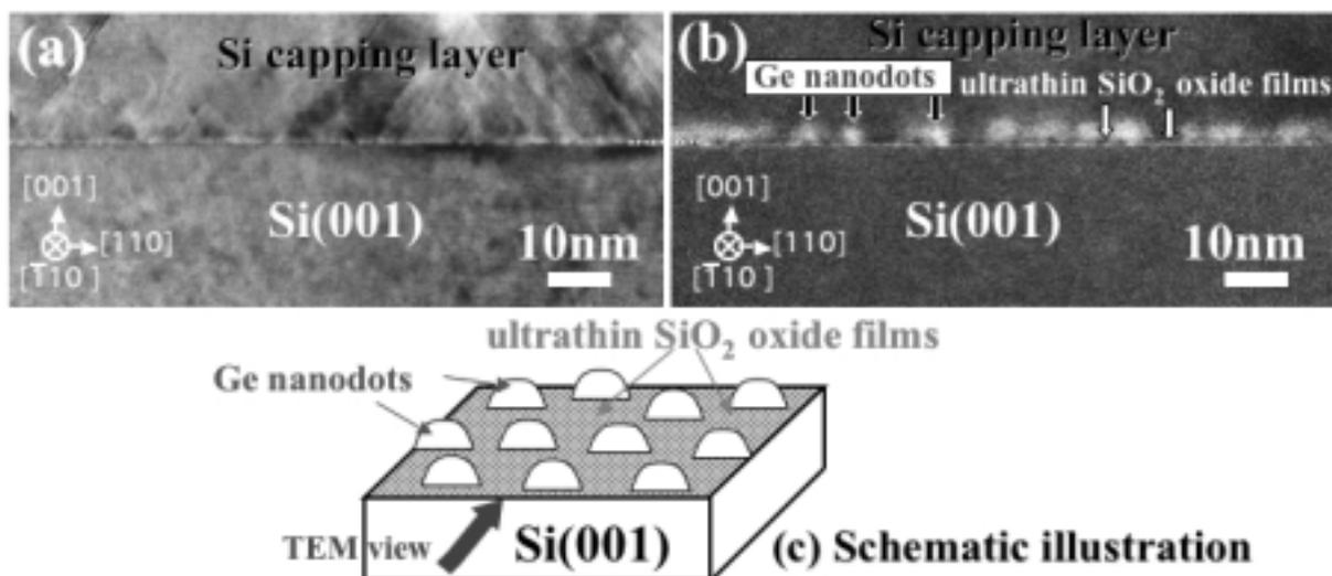
FIG. 1: (a) Conventional TEM image, (b)  $C_s$ -corrected HADF-STEM image of poly-Si cap layer/Ge-nanodots/silicon-oxide films/Si(001), and (c) bird-view illustration.
