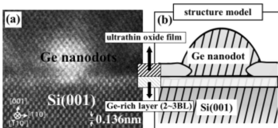
FIG. 2: (a)  $C_s$ -corrected high-resolution HAADF-STEM image revealing the details of the interface structures, (b) a newly proposed structure model of Ge nanodots grown on slightly oxidized Si surfaces.
