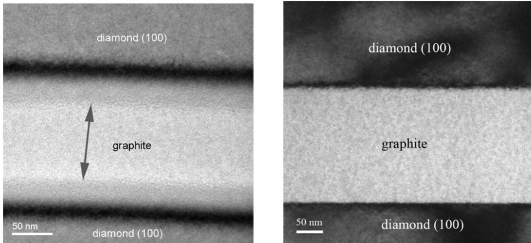
FIG 2: TEM images of the damage layer in diamond after annealing at 550°C (a) and 1260°C (b).
