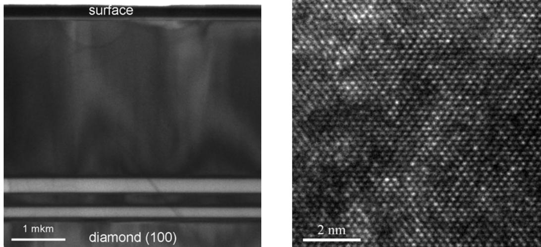
FIG. 1: a) cross-sectional image of diamond with two damage layer; as implanted b) HREM image of thin 'sandwiched' diamond layer.
