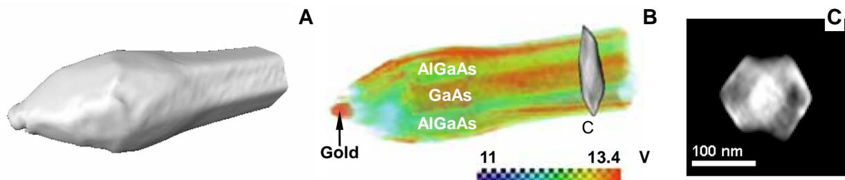
*Fig. 2 3D Potential of a GaAs/AlGaAs nanorod reconstructed from holographic tilt series.*
