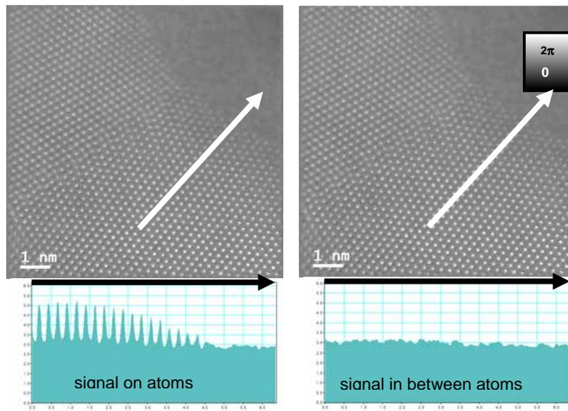
*Fig. 1 Phase image of a gold crystal reconstructed from a XFEG-hologram.*
