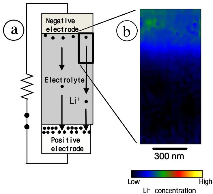
FIG. 2. In-situ measurement of Li-ion distribution when the two electrodes were connected; (a) schematic of the experimental setup, and (b) phase map. The electric potential in (b) is almost flat in the vicinity of the negative electrode.
