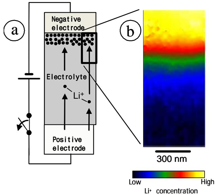
FIG. 1. In-situ measurement of Li-ion distribution after charging; (a) schematic of the experimental setup, and (b) phase map. The yellow region in (b) indicates high electric potential from positive Li ions in the vicinity of the negative electrode.
