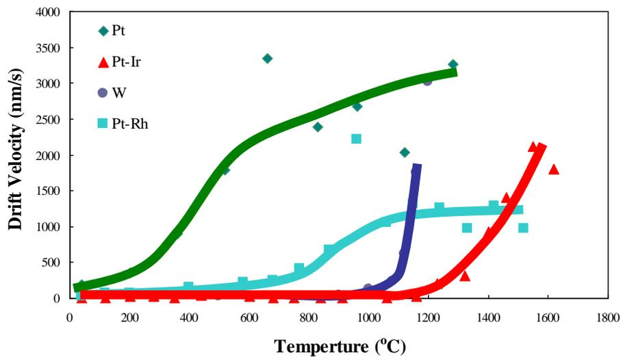
Fig. 3: graph of relationship between temperature and drift velocity of each wire coils
