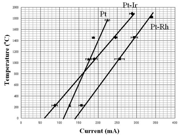
Fig. 2: graph of relationship between current and temperature of each wire coils
