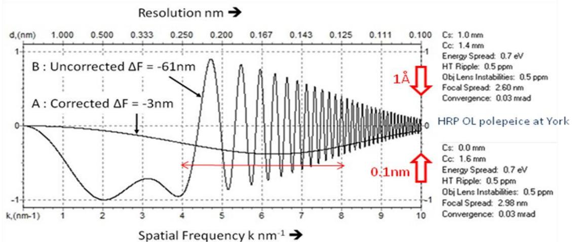
Fig. 2 Contrast transfer function calculated for the corrected instrument (A) and for the uncorrected native York 200kV microscope (B).
