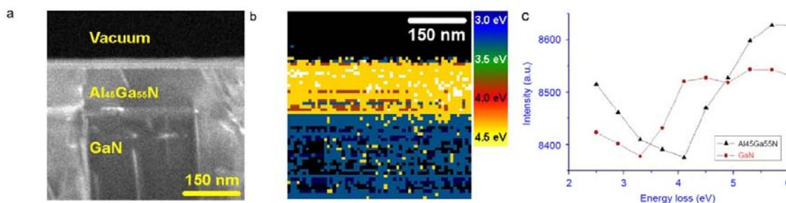
FIG. 2. Band-gap mapping of the same  $\text{Al}_{45}\text{Ga}_{55}\text{N}/\text{GaN}$  structure. (a) A raw EF-STEM micrograph integrated from 2.5 to 6 eV. (b) Band-gap mapping with the corresponding energy labeled on the right. (c) Extracted spectrum profiles of  $\text{Al}_{45}\text{Ga}_{55}\text{N}$  and GaN. Detailed experimental procedure is described in Ref. [3].
