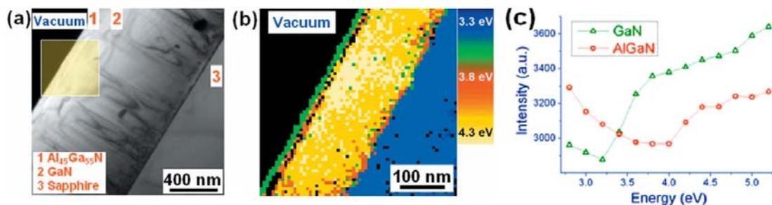
FIG. 1. (a) The sum of all energy-filtered images from 2 to 32 eV shows the  $\text{Al}_{45}\text{Ga}_{55}\text{N}/\text{GaN}/\text{sapphire}$  structure. (b) Band-gap map of the region marked in (a) with a pixel size of about 7.2 nm, corresponding band-gap values can be read from the legend. (c) Electron energy-loss spectra extracted from the 3D EFTEM stack indicating a bandgap difference of about 0.8 eV. [2].
