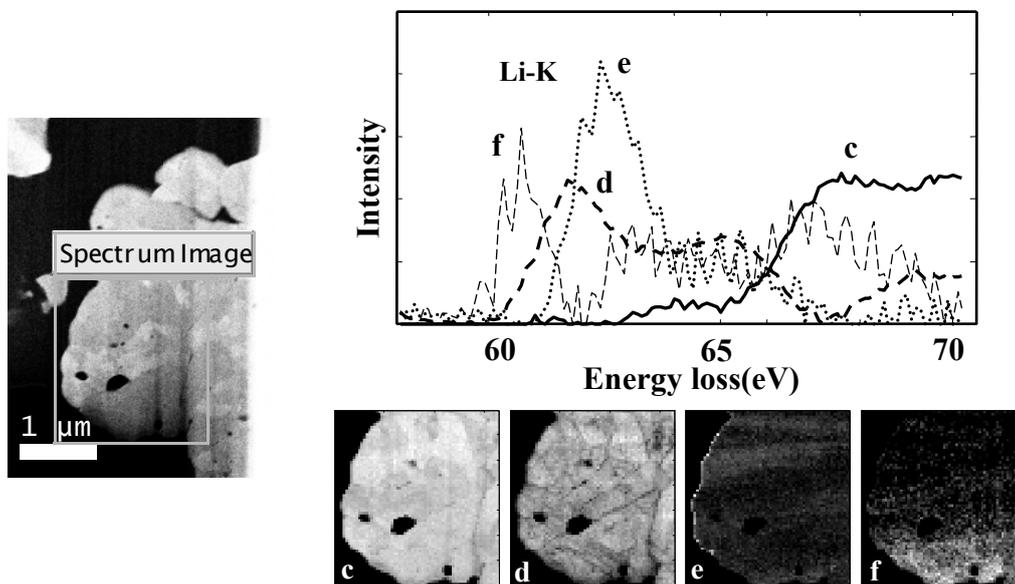
Fig. 2 Result of MCR for Li-K ELNES after 500 cycling at 70°C
