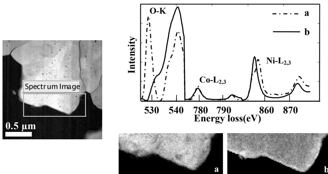
Fig. 1 Result of MCR for O-K, Co-L<sub>2,3</sub>, Ni-L<sub>2,3</sub> ELNES after 500 cycling at 70°C (Spatial distributions of resolved components and pure spectral profiles are shown on the right side.)
