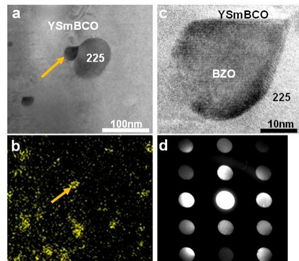
FIG. 4. (a) a BZO particle in YSmBCO indicated by an arrow, (b) Zr-map correspond to the region (a), (c) higher magnification image of the BZO in (a), and (d) nano-beam diffraction pattern along the BZO [110] zone axis for the BZO in (c).
