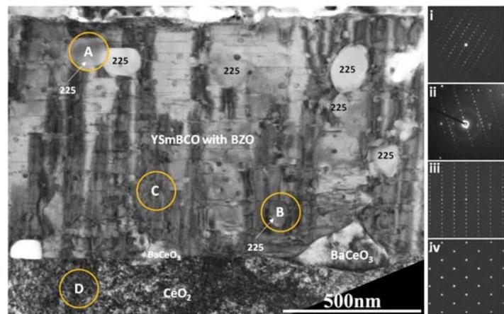
FIG. 2. Cross-sectional electron micrograph of the YSmBCO coated conductor with (i)-(iv) selected area diffraction patterns corresponding to the region of A-D in the micrograph.
