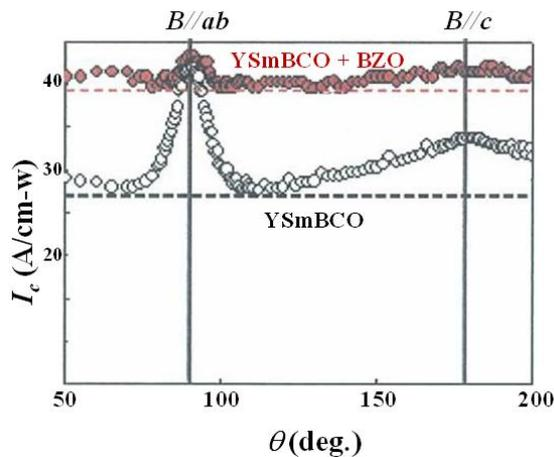
FIG. 1. The field angular dependence of  $I_c$  of YSmBCO coated conductors with and without BZO at 77 K under a magnetic field of 1 T.
