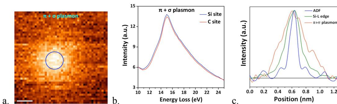
FIG 3. (a) Plasmon map (11-18 eV) showing localized enhancement of the  $\pi + \sigma$  plasmon at a substitutional Si atom. (b) Comparison of the graphene  $\pi + \sigma$  plasmon spectra, extracted from the Si atomic site and from the carbon site. (c) Comparison of the delocalization of the ADF signal, the Si-L edge signal, and the enhanced plasmon intensity from the Si atom. Scale bar: 0.2 nm. (a) reproduced from Ref [6].
