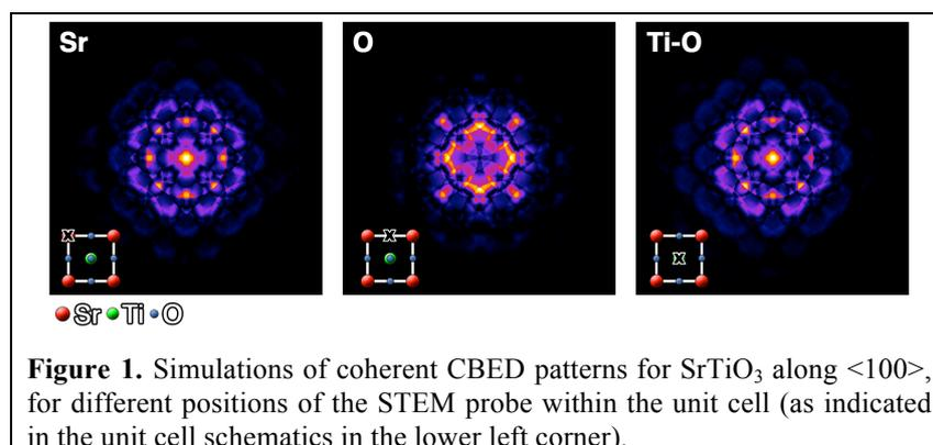
A PACBED pattern is formed through incoherent averaging of CBED patterns over many probe positions. The fine detail resulting from coherent interference is then lost, but better count rates and a reduced sensitivity to instability are obtained. The
