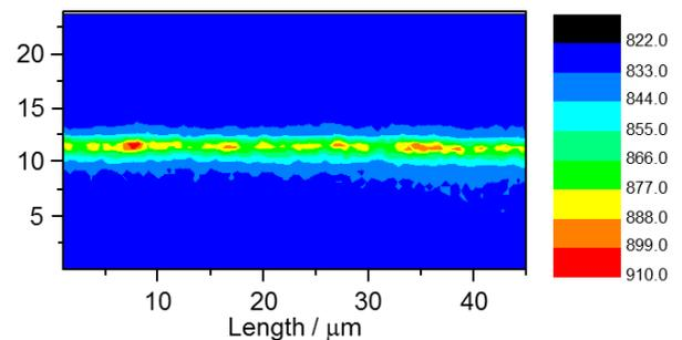
FIG. 3. Intensity map of the ruby induced luminescence at 694.2 nm obtained by using confocal micro-luminescence spectroscopy. The distribution of the luminescence was detected along the grain boundary.
