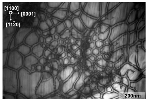
FIG. 4. A BF-TEM image of the secondary phase-alumina matrix interface observed from [1100] plan-view direction. The formation of a complex misfit dislocation network structure was observed.
