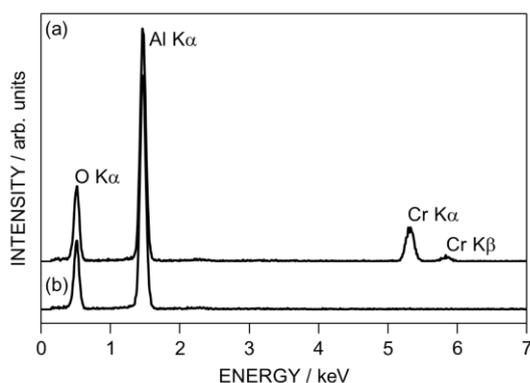
FIG. 2. TEM-EDS spectra obtained (a) at an area in the secondary phase and (b) at an area 3 nm outside the secondary phase-alumina matrix interface.
