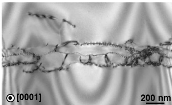
FIG. 1. A BF-TEM image of the grain boundary observed from [0001] direction. The formation of an approximately 200 nm width secondary phase can be seen.
