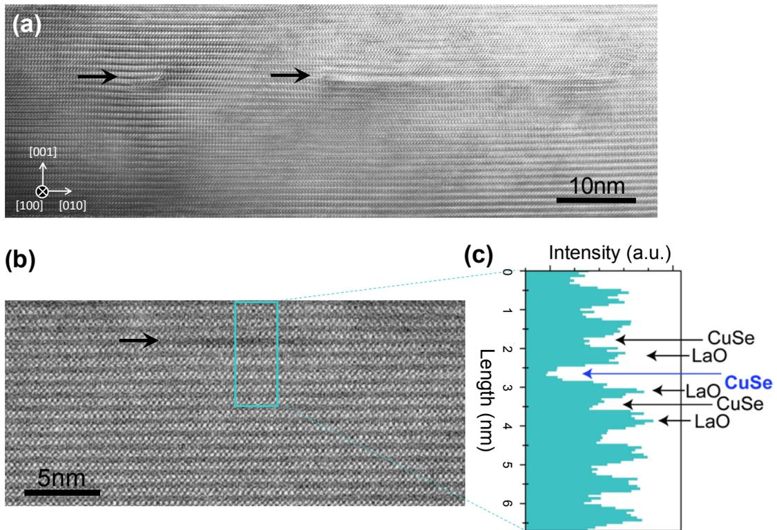
FIG. 1. (a) HRTEM image of LaCuOSe:Mg thin film observed along [100] zone axis. (b) Magnified HAADF-STEM image around a planar defect. Horizontal black arrows in the images indicate planar defects. (c) Intensity profile taken from the square region in the STEM image.
