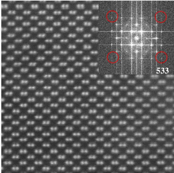
FIG.1 HAADF image of Si  $\langle 110 \rangle$  obtained by Titan cube operating at 300 kV. ADF detector spanning 38.4–191.8 mrad. The sample has been made by FIB at low accelerating voltage 2kV. Fourier transform showing the presence of the (533) spacing at 0.083nm, confirming the less than 0.1nm information transfer.
