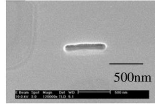
FIG.2 SEM image of surface crystal defect.
