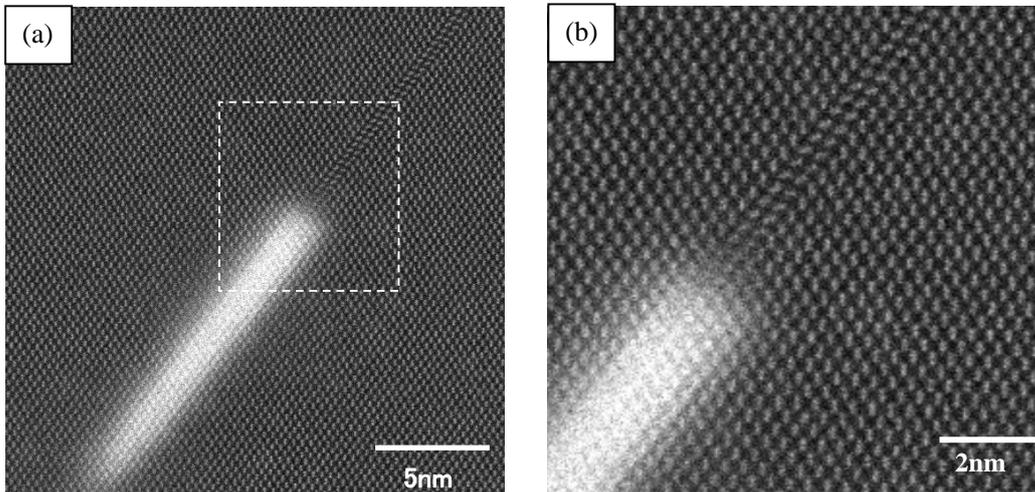
FIG.4 (a): HAADF image of the silicon wafer / epitaxial silicon layer interface. The bright contrasts are Ni silicide. The twin defect was also observed. (b): Enlarged image of dotted line area in (a). The twin defect has been generated from Ni silicide.
