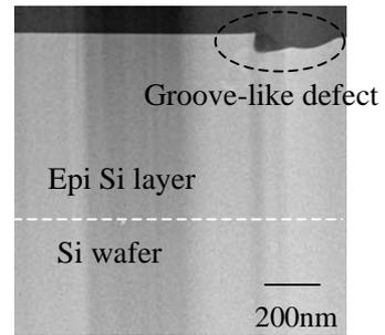
FIG.3 Cross-sectional image of groove-like defect.
