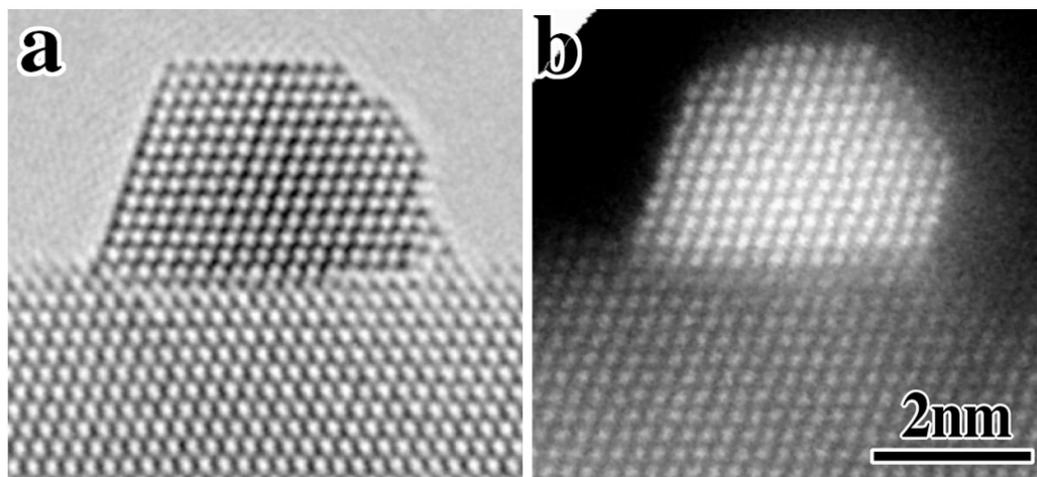
FIG. 1. HRTEM image of Au particle on NiO(111) surface (a) and HAADF-STEM image(b).
