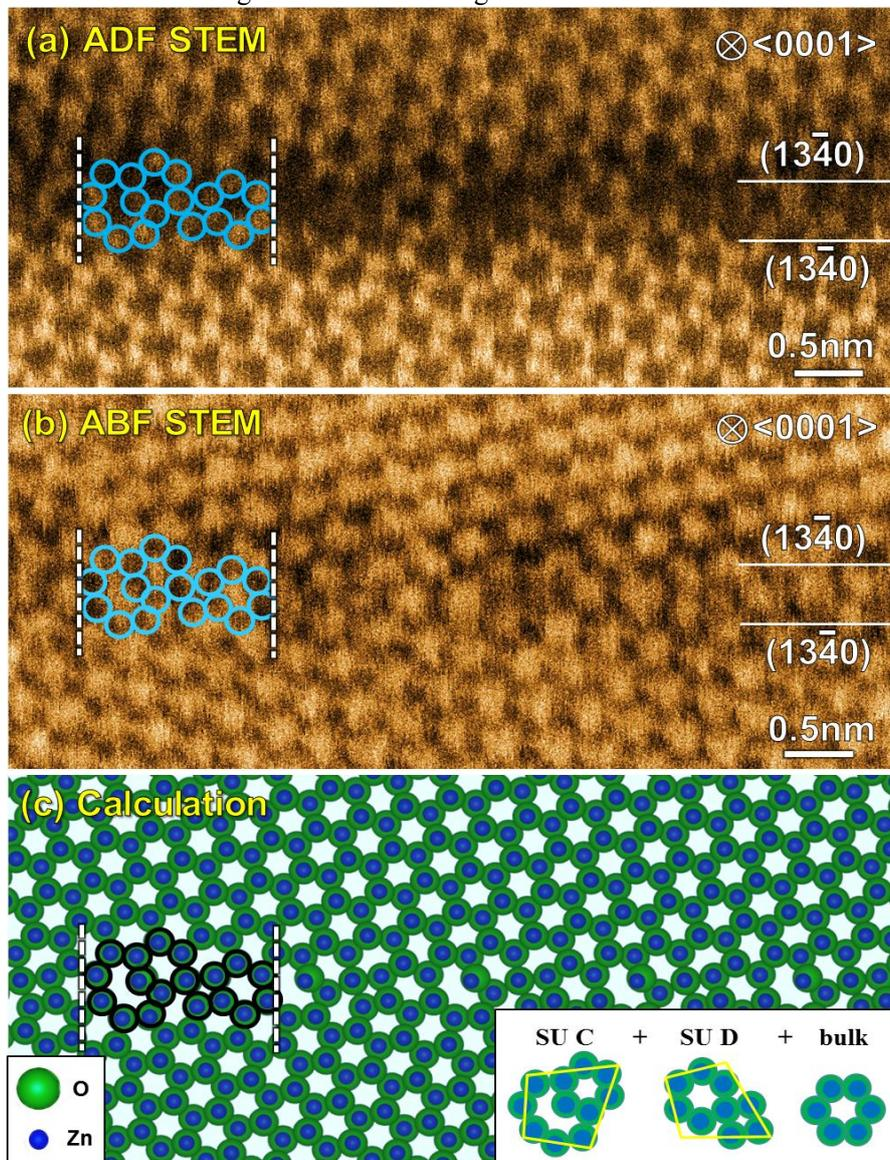
FIG. 2. (a) Annular dark-field and (b) annular bright-field STEM image of ZnO GB. (c) Calculated GB structure model with an inset showing the combination of SUs at the GB. Here, SUs (C+D+bulk) forms a single structural period at the GB.
