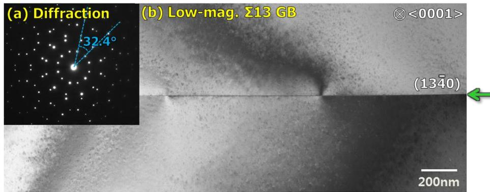
FIG. 1. (a) Diffraction pattern taken from the region including both crystals and (b) low magnification TEM image of ZnO  $\Sigma 13$ GB.
