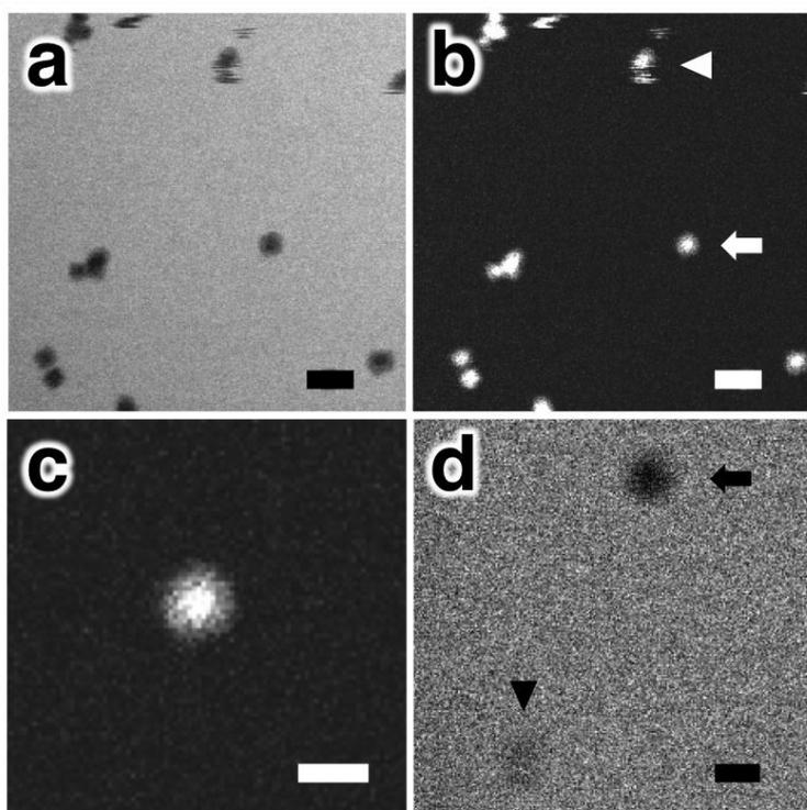
**Figure 1** (a&b) *In situ* bright field and dark field STEM images of a suspension of ferritin molecules in a buffered saline solution. The white arrowhead points to a ferritin molecule that moved during acquisition. c) Magnified view of ferritin molecule indicated by white arrow in (b) depicting both the outer protein shell and more dense (brighter) inner iron oxide nanoparticle. d) *In situ* bright field STEM image of ferritin and apoferritin. Scale bars are 10 nm.
