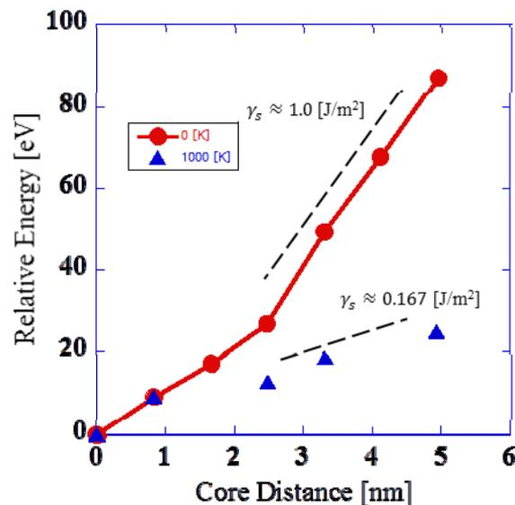
FIG. 1. Relative energy of the system as a function of distance between partial screw dislocations.
