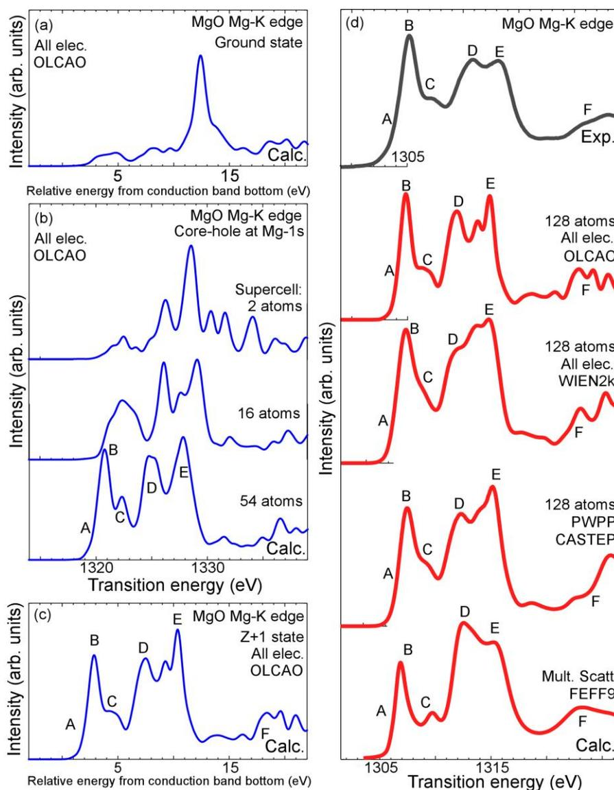
Fig.1 Calculated Mg-K edge of MgO at (a) ground state, (b) final state with different sizes of supercell, and (c) Z+1 state. (d) Experimental and calculated Mg-K edge of MgO. The calculations were performed at the final state with sufficient calculation size using the all-electron (All elec.) OLCAO method, WIEN2k code, FEFF9 code, and plane wave based pseudopotential (PWPP) method implemented in CASTEP code.
