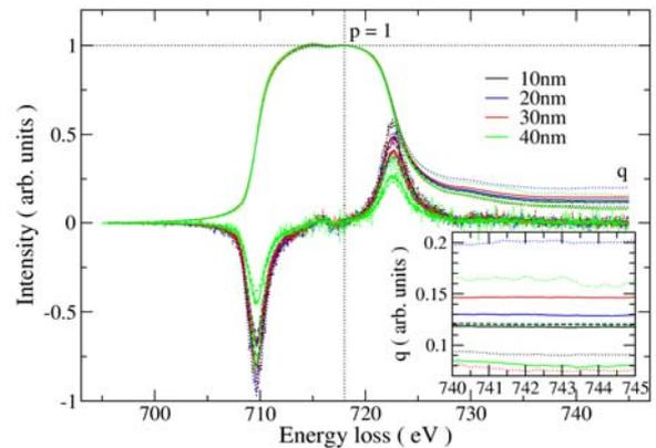
FIG. 2. EMCD spectra and their energy integrals of bcc iron crystal at 4 different thicknesses obtained by the MCR method.
