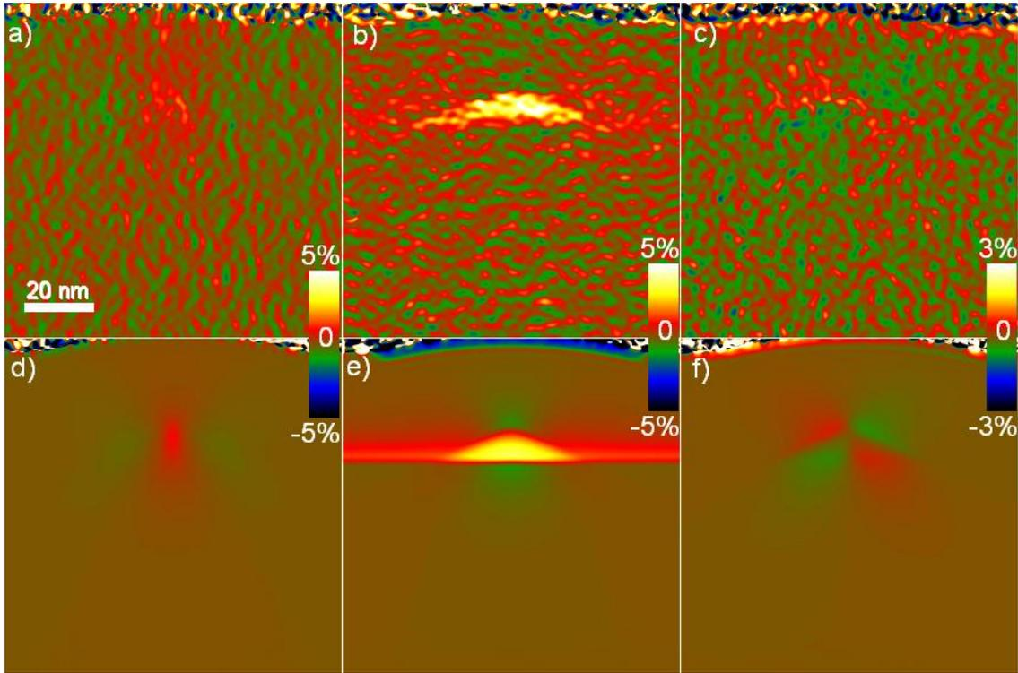
FIG. 1. Measurements of the strain relative to GaAs lattice obtained by dark-field electron holography (a), (b), (c) and by geometric phase analysis of the image generated by FEM (d), (e), (f) of the In(Ga)As QD almost totally embedded within a TEM lamella: (a), (d) in-plane strain,  $\epsilon_{xx}^{GaAs}$ ; (b),(e) out-of-plane strain,  $\epsilon_{zz}^{GaAs}$ ; (c), (f) shear strain,  $\epsilon_{xz}^{GaAs}$ .
