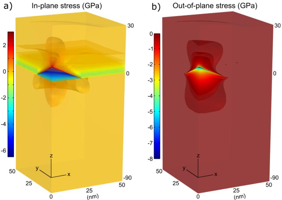
FIG. 2. 3D stress distributions modeled by finite-element method (FEM): (a) in-plane stresses; (b) out-of-plane stresses.
