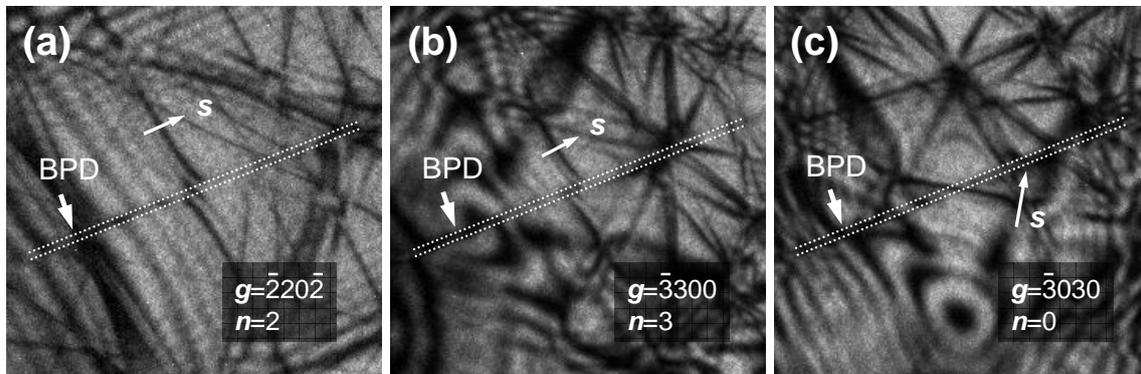
Fig. 3 Bright-field LACBED patterns obtained around the BPD containing a perfect area.  $s$ ,  $g$  and  $n$  denote the direction of excitation error, the reciprocal lattice vector of the reflection and the number of nodes, respectively.
