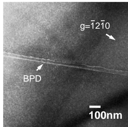
Fig. 2 A  $g$ - $3g$  WBDF image using  $\bar{1}2\bar{1}0$  reflection of the 4H-SiC containing the BPD. The BPD is dissociated into partial dislocation pairs.
