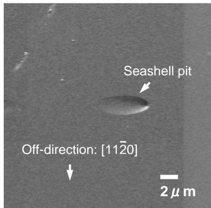
Fig. 1 Seashell pit image on a (0001) 4H-SiC substrate after KN etching. The seashell pit is perpendicular to the  $[11\bar{2}0]$  (off-) direction.
