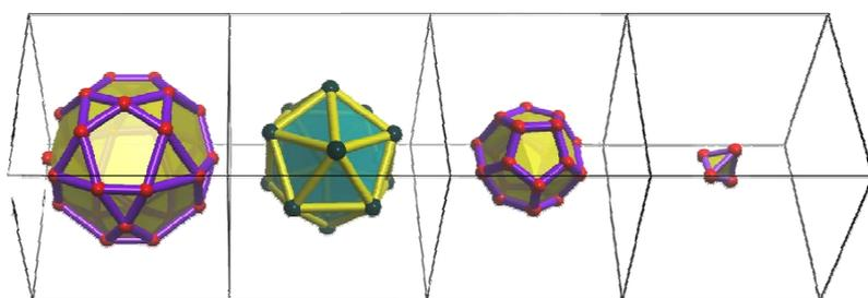
FIG. 1. Schematic illustration of a Tsai-type icosahedral cluster.
