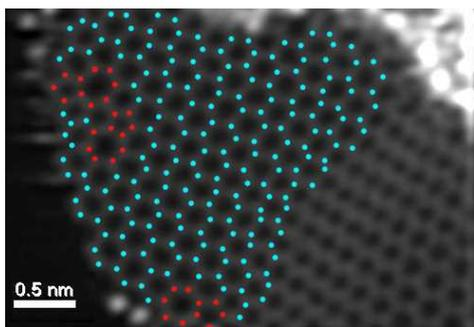
FIG. 1. Annular dark-field STEM image of ultramicroporous carbon showing a graphene layer with 5- and 7- membered defects. [3].
