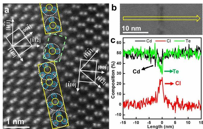
FIG. 4. (a) Structure of a  $\Sigma 9$  GB. (b) Composition profile showing significant Cl enrichment and Te depletion at the GB plane in (c). Blue and yellow circles indicate Cd and Te columns, respectively [6].
