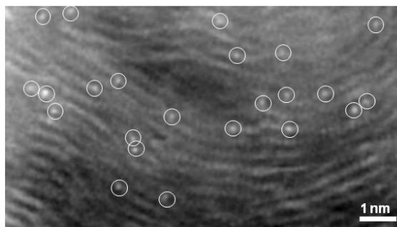
FIG. 2. Annular dark-field STEM image of a Nb-C catalyst showing single Nb atoms trapped in graphitic carbon [4].
