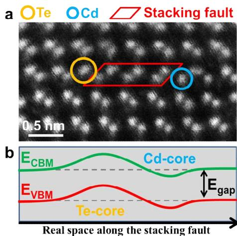
FIG. 3. (a) Z-contrast image shows Cd and Te single atom columns (blue and yellow circles) at two ends of an intrinsic stacking fault (red box). (b) Sketch map shows band bending along the stacking fault. [5].
