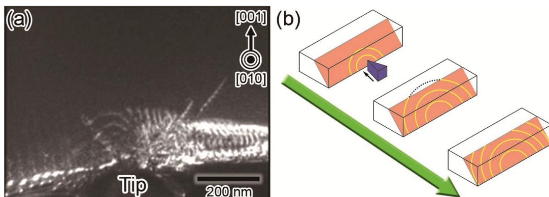
FIG. 1. (a)Dark-field TEM image during the TEM nanoindentation to SrTiO<sub>3</sub> single crystal and (b)Schematic illustrations of introduction mechanisms of lattice dislocations
