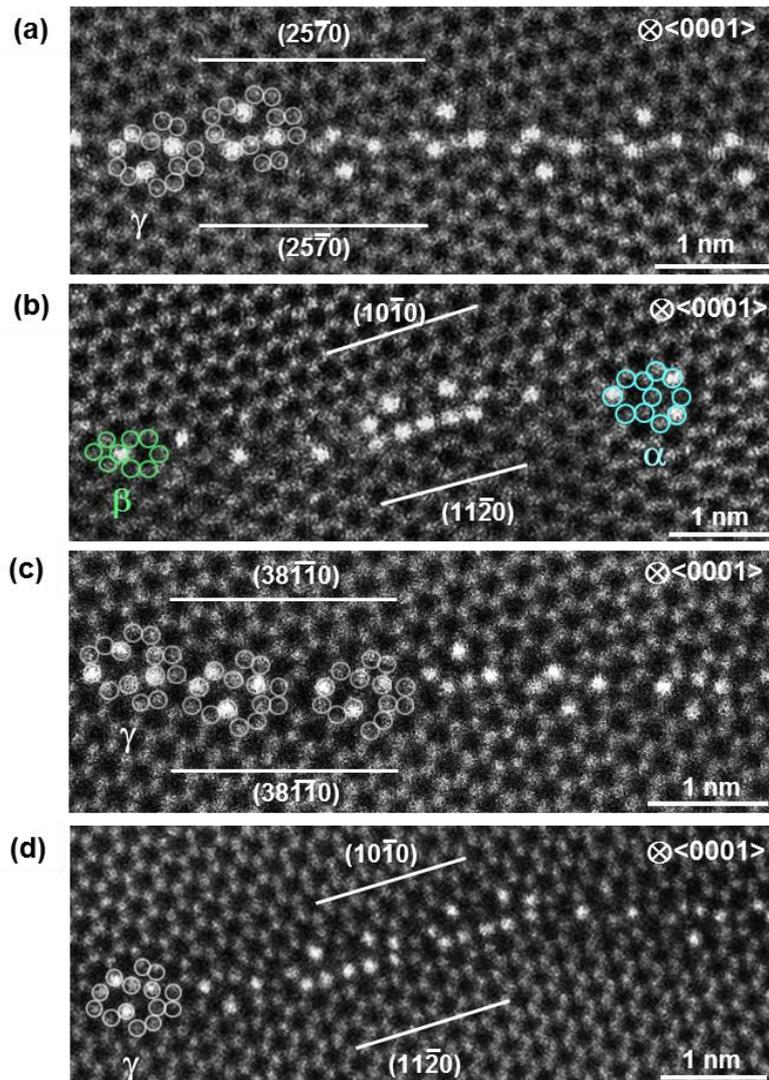
**Fig. 1.** HAADF-STEM images of the Pr-doped ZnO  $27.8^\circ$   $[0001]$  tilt GB (a) in the  $(25\bar{7}0)$  boundary plane region and (b) in a facet. HAADF-STEM images of the Pr-doped ZnO  $30.0^\circ$   $[0001]$  tilt GB (c) in the  $(38\bar{1}10)$  boundary plane region and (d) in a facet. Brightest contrast indicates the location of Pr. SUs ( $\alpha$ ,  $\beta$ , and  $\gamma$ ) are indicated by sets of circles.
