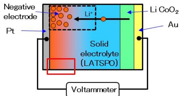
FIG. 1. Schematic of the model battery sample used in the experiments. An area corresponding to that enclosed by the red rectangle was observed by electron holography and SR-EELS.
