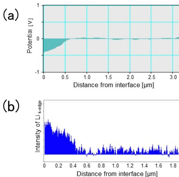
FIG. 2. Results from (a) *in situ* electron holography and (b) SR-EELS at the negative electrode side, showing the electric potential distribution and lithium concentration, respectively, as a function of distance. The negative electric potential on the left-hand side in (a) is consistent with the excess Li content in (b) in the *in situ* formed negative electrode even after different numbers of cycles.
