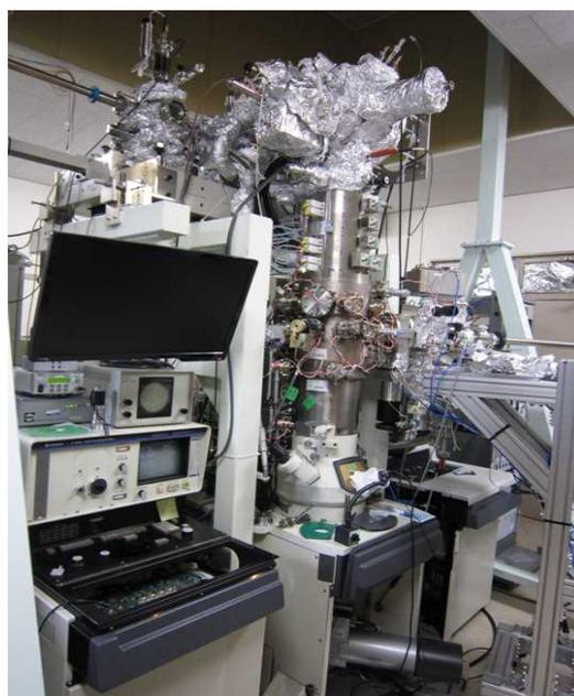
Fig. 2 : Photo of 30 kV spin-polarized/pulsed and holographic TEM driven by Ti-pulsed laser.
