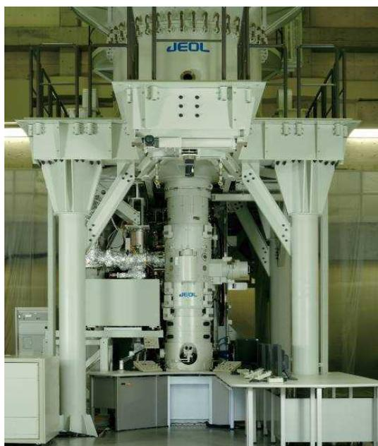
Fig. 1 : External view of 1 MV RSHVEM with a high-speed beam-blanking system.
