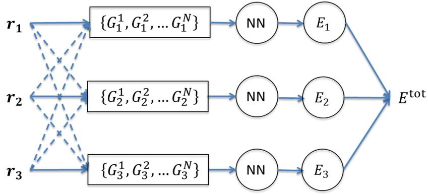
Fig. 1 Structure of NNP as applied to a system containing three atoms, where  $r_i$  and  $G_i^j$  denote the position and  $j$ th symmetry function of  $i$ th atom, respectively. The neural network approximates the complex function of the energy of  $i$ th atom,  $E_i$ , using the symmetry functions. The total energy  $E^{\text{tot}}$  is computed as the sum of atomic contributions  $E_i$ .
