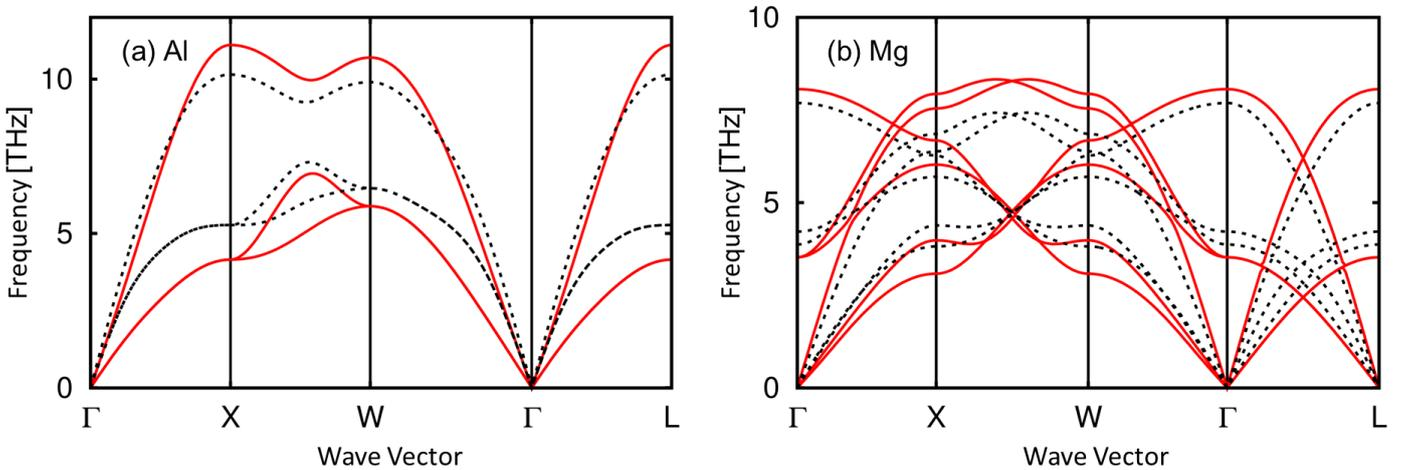
Fig. 3 Phonon dispersion curves obtained by NNP (red solid lines) and DFT (black broken lines) for (a) Al and (b) Mg.
