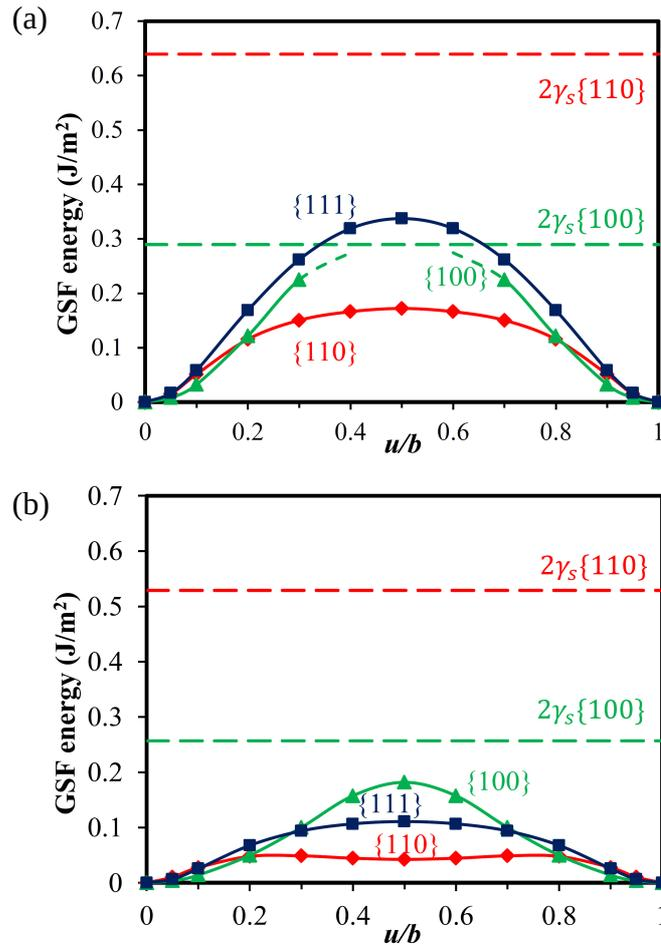
Fig.1. GSF energy curves for (a) NaCl and (b) AgCl, as a function of the displacement  $u$  divided by the Burgers vector. These results are for the slip direction of  $\langle 110 \rangle$ .
