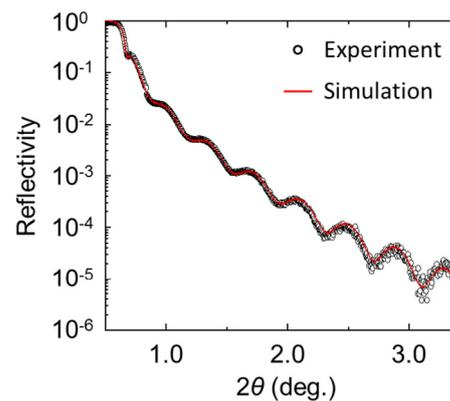
Fig. 2. X-ray reflectivity of a  $\text{Sn}_2\text{Nb}_2\text{O}_7$  thin film and a simulated profile with a thickness of 21 nm, roughness of 0.8 nm, and density of  $5.5 \text{ g/cm}^3$ .
