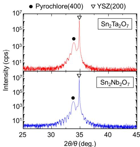
Fig. 1.  $2\theta$ - $\theta$  XRD profiles of  $\text{Sn}_2\text{Nb}_2\text{O}_7$  and  $\text{Sn}_2\text{Ta}_2\text{O}_7$  thin films.
