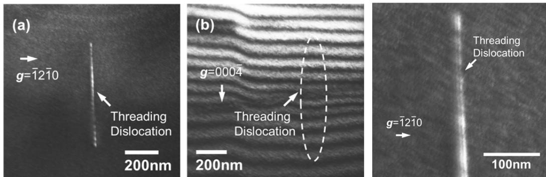
Fig. 1 Dark-field images under the  $g/3g$  weak-beam condition of the threading dislocation which exists below the small hexagonal pit. (a)  $g=\bar{1}2\bar{1}0$ , (b)  $g=000\bar{4}$ .
