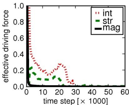
FIG. 2. Time evolution of the driving force for the variant selection. Red dotted, green broken and black solid lines represent interface, strain and magnetic contributions, respectively.
