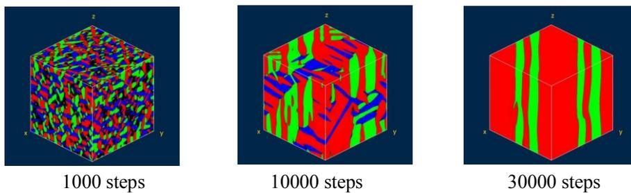
FIG. 1. Time evolution of microstructure under an external magnetic field of 6 T. Red, green and blue regions represent the variants of  $L1_0$  phase of which  $c$ -axis is along  $x$ ,  $y$  and  $z$  direction, respectively.
