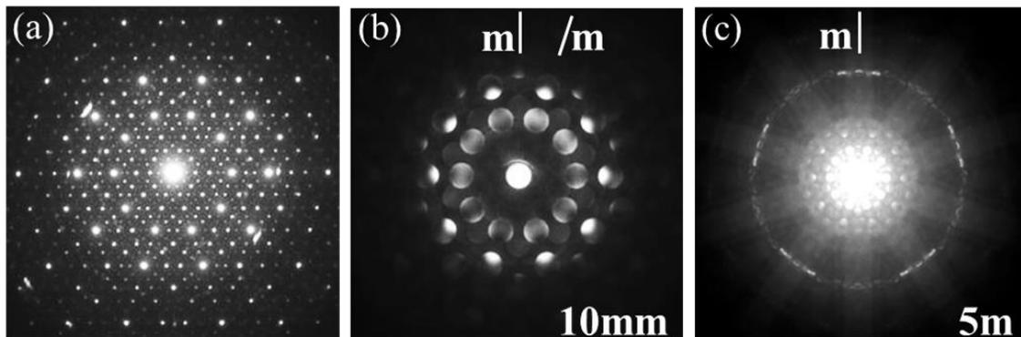
Figure 1. NBD and CBED patterns of ZnFeSc iQC at an incidence parallel to the fivefold axis. The NBD pattern (a) and the CBED pattern formed by ZOLZ reflections (b) and HOLZ reflections (c).
