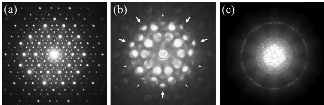
Figure 2. NBD and CBED patterns of ZnSc PD type iQC at an incidence parallel to the fivefold axis. The NBD pattern (a) and the CBED pattern formed by ZOLZ reflections (b) and HOLZ reflections (c).
