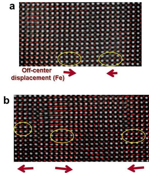
FIG. 2. Plots of off-center Fe displacement vectors. (a) Low-strain region. (b) High-strain region. The displacement vectors are superimposed on each STEM image, showing much larger magnitudes in the high-strain region. For direct comparison and better visualization, thick red arrows are included to represent the direction of the Fe displacement vectors in the domains denoted by yellow ovals. Antiparallel polarizations of the dipoles between domains are noted.
