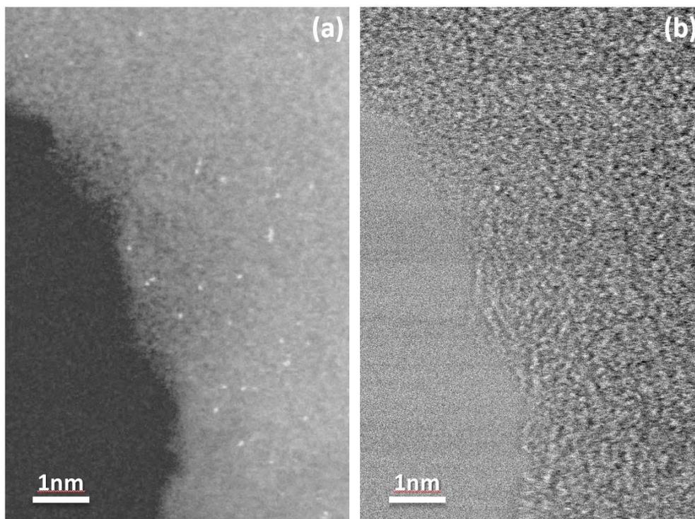
Figure 1 (a) HAADF and (b) BF image of Er doped glass fiber.
