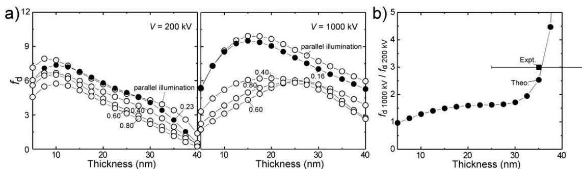
FIG. 3. (a) Theoretical  $f_d$  with  $V = 200$  and  $1000$  kV. Numbers inset are  $\phi_{\text{col}}$ , represented by EELS aperture radii in  $g$ . Filled circles are results with the experimental  $\phi_{\text{col}}$ . (b) Theoretical and experimental ratios of  $f_d$  between  $V = 200$  and  $1000$  kV.
