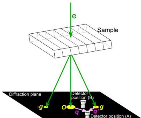
FIG. 1. Set-up of intrinsic EMCD measurement using the sample crystal as a beam splitter.  $q$  and  $q'$  are scattering vectors for direct and diffracted beams falling into the EELS detector placed at (A).
