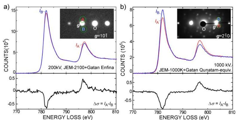
FIG. 2. Experimental Co- $L_{2,3}$  ELNES collected at two different EELS aperture positions (A), (B). Two sets of results obtained by using different TEM-EELS systems with different acceleration voltages are shown.
