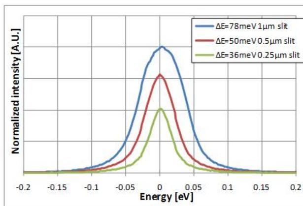
FIG. 1. Intensity profiles of zero-loss peaks for the slit of 1  $\mu\text{m}$ , 0.5  $\mu\text{m}$  and 0.25  $\mu\text{m}$  obtained with 0.1 seconds acquisition at 200 kV.
