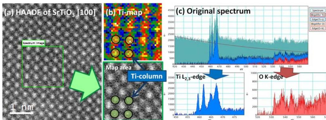
FIG. 3. (a) Raw HAADF-STEM image of  $\text{SrTiO}_3$  [100] obtained with 112 pA probe current and 146 meV energy resolution at 200 kV, (b) Ti map of  $\text{SrTiO}_3$  [100], (c) Original spectrum with 0.05 sec. acquisition time and background-subtracted spectra of Ti  $L_{2,3}$ - and O K-edges.
