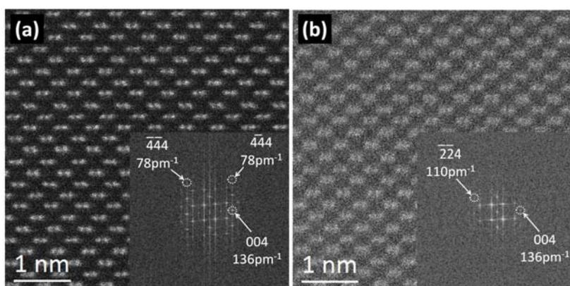
FIG. 2. Raw HAADF-STEM images of Si [110] with different setting of monochromator at 200 kV and their Fourier transforms. (a) Energy spread of 294 meV using 4  $\mu\text{m}$  slit with 12 pA probe current and 38  $\mu\text{s}/\text{pixel}$  scan speed, (b) Energy spread of 36 meV using 0.25  $\mu\text{m}$  slit with 0.8 pA probe current and 100  $\mu\text{s}/\text{pixel}$  scan speed.
